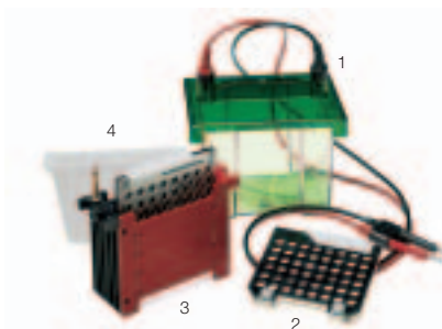
Fig. 1.5. The Mini Trans-Blot cell. 1, buffer tank and lid; 2, gel holder cassette; 3, electrode assembly; 4, Bio-Ice™ cooling unit.
